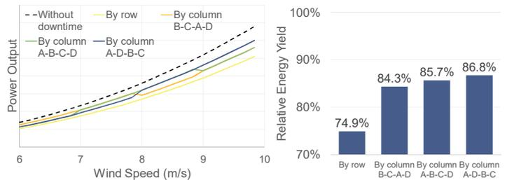
Figure 4: (left) Power produced in different maintenance schedules against a wind speed linearly increasing over time; (right) energy yield produced by various maintenance schedules compared to energy yield without downtime. Order of shutdown by column is indicated where "A-B-C-D" is in order from West to East.
