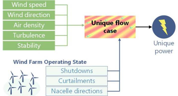
Figure 1: The factors that WakeBlaster considers in the simulation of 10-minute mean power
