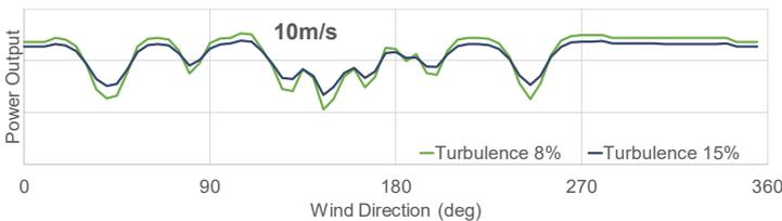
Figure 3: WakeBlaster simulated power of a heavily waked turbine. Higher turbulence intensity decreases the strength of the wakes but also decreases output at the knee of the power curve.
